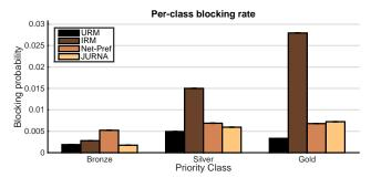
Fig. 7. Average blocking rate (probability of active client blocking).
