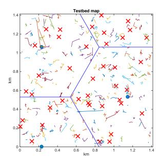
Fig. 2. BS positions in a 2  $\text{km}^2$  map. 3G and 4G are co-located in the centre of each cell, while WiFi APs are placed uniformly (x). The mobility trajectories of the clients are also shown.
