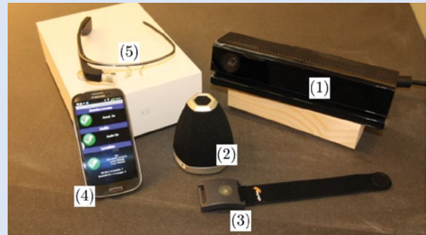
Figure 9 Sensors available in the social sensing lab. (1) Kinect V2, (2) Microcone, (3) Q-Sensor, (4) Android smartphone, (5) Google Glass.
