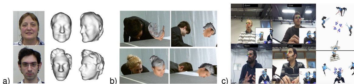
Figure 14: Attention analysis - Accurate and robust 3D head and gaze tracking. a) Example of online reconstructed heads. b) Tracking results in adverse conditions (UBI Impressed registration desk set-up). c) Gaze coding in multi-party interactions: Heads are tracked, eye localized and aligned before inferring gaze and attention towards people or other semantic labels (all information analysed in 3D).
