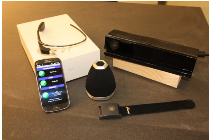
Figure 12: Sensors available in the social sensing lab. Kinect V2, Microcone, Q-Sensor, Android smartphone, Google Glass.
