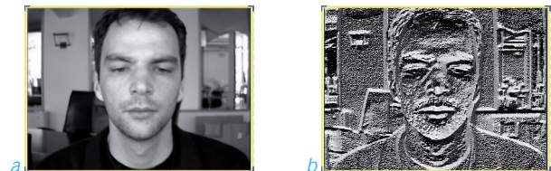
Figure 9: Illustration of the LBP feature map (b) for the original image (a).
