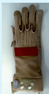
The CyberGlove was developed to record and reproduce the daily movements of the hand.
