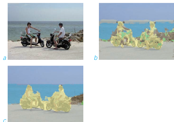
Figure 7: Our recurrent scene parser over original image (a) segments the image as shown in (b). Due to its recurrent nature, it can be fed again with its own prediction (b) and the original image (a), which leads to (c): most mistakes are corrected.
