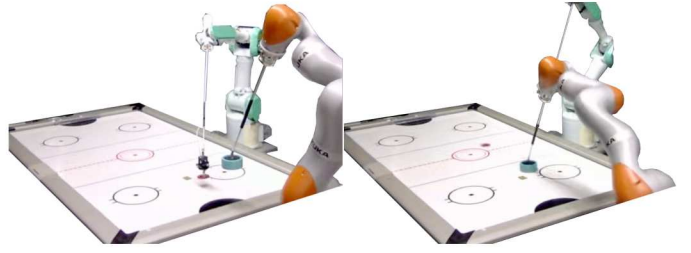
Fig. 6. The automated experimental setup consists of a robot placing the puck at a pre-defined grid of positions (left image). After releasing the puck, the KUKA robot executes the shooting policy (right image). We measure the speed of the puck at the goal line and whether the puck hit the goal as quality metrics.
