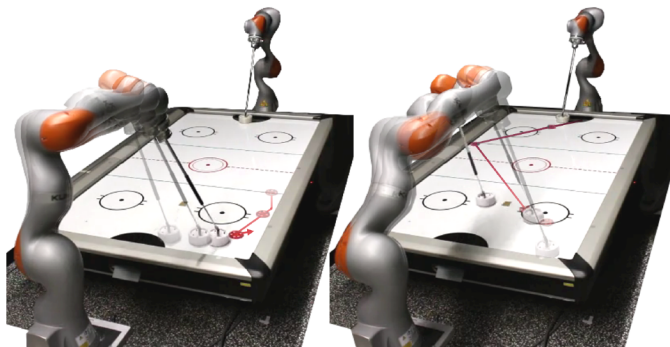
Fig. 1. The proposed control framework enables our robot to autonomously play matches of air hockey. The dynamic game requires the robot to predict puck trajectories, plan the best contact, and coordinate its joints to generate high velocities without hitting a wall or lifting the mallet from the table.
