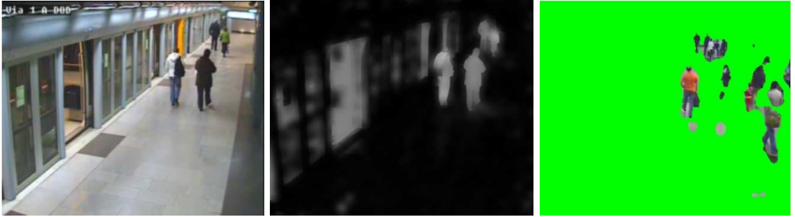
Fig. 4: Example of background subtraction processing, and issues for human detection. Foreground regions may contain other objects (e.g. cars for outdoor scenes). Specular reflection and cast shadow can generate background false alarms. People might only be partially visible (e.g. split into multiple blobs), and a given blob may contain several people. Also, there might be ghosts when people are integrated in the background model and then leave the scene.
