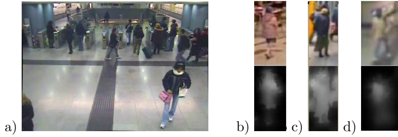
Fig. 1: (a) Example of surveillance metro image. (b)-(d) Appearance and foreground samples from other data: (b) the person is camouflaged by the background, while foreground is more precise; (c) and (d) foreground is noisier but appearance remains discriminative. More examples can be found in Fig. 3.
