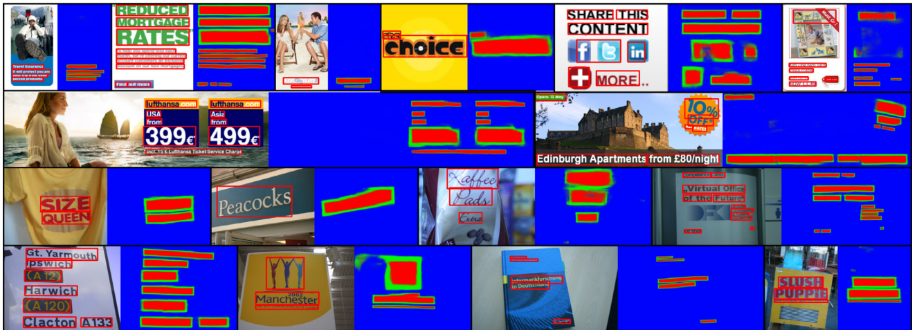
Fig. 7. Illustration of STSN output on ICDAR 2011 (top rows) and ICDAR 2013 (bottom rows).
