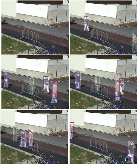
Figure 6: Frames 1,78,155,168,211,295 from an experimental run of seq4 . Estimated configurations are shown as colored boxes where color corresponds to object ID, and the ground truths as shaded areas.
