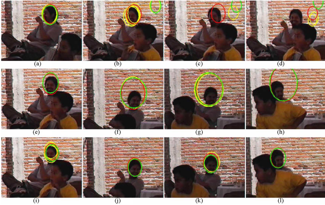
Fig. 8. Head tracking 1 (colors in parentheses refer to the electronic version of the paper). First row: Shape-based tracker M1. Second row: Shape-based tracker M2. Third row: Shape-based tracker M3. In dark gray (red), mean state; in medium gray (green), mode state; in light gray (yellow), likely particles. (a) t_1 . (b) t_{10} . (c) t_{11} . (d) t_{13} . (e) t_{12} . (f) t_{24} . (g) t_{45} . (h) t_{63} . (i) t_{12} . (j) t_{24} . (k) t_{45} . (l) t_{63} .
