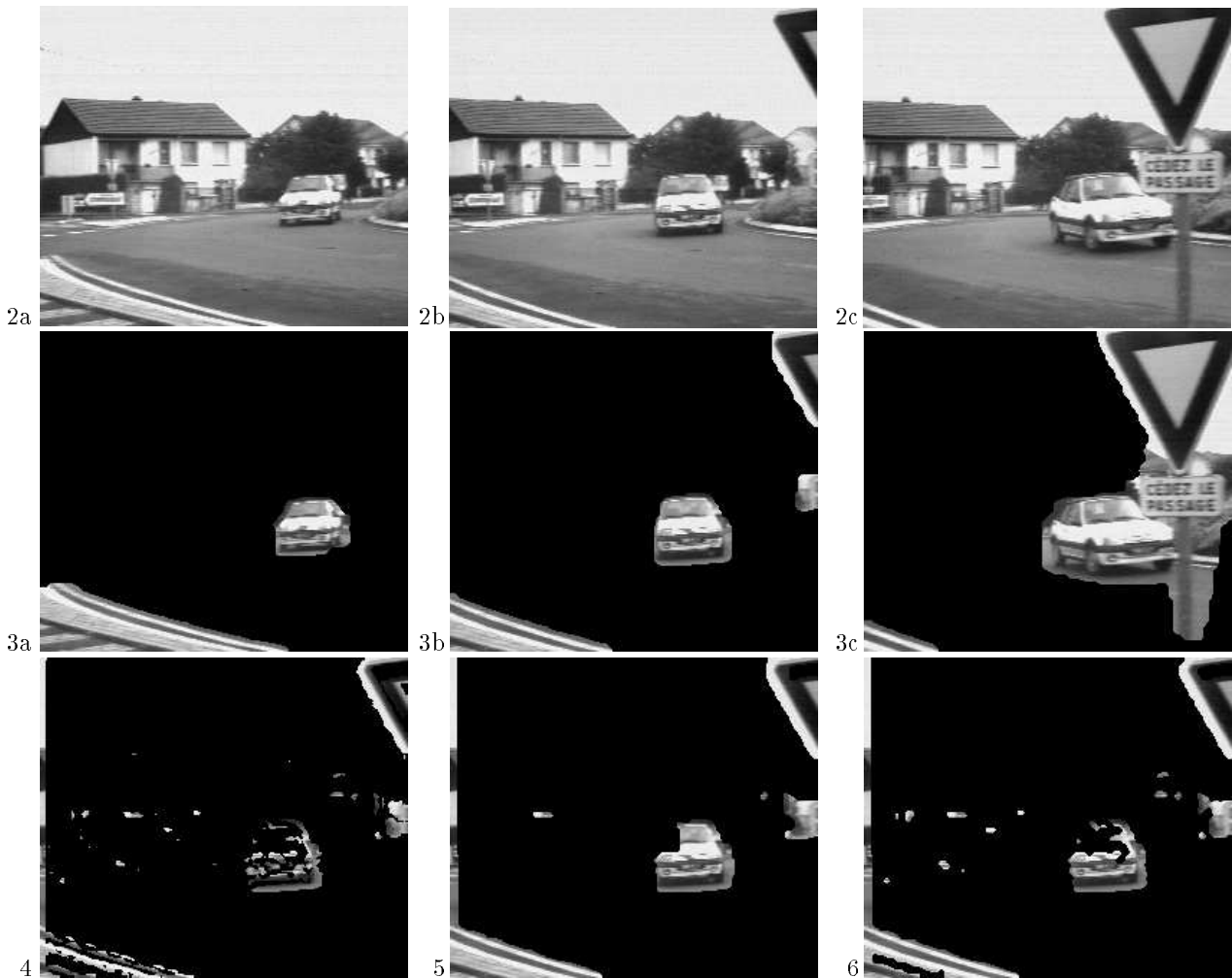
Fig. 2a, 2b and 2c : three images of the “roundabout” sequence at time t_{57} , t_{62} and t_{67} . Fig. 3a, 3b and 3c : results with parameter values ( \alpha = 66 ): \delta = 1.0 , \beta_{\text{diff}} = 40 , \beta_m = 4 , \tilde{\beta}_{\text{diff}} = 27 , G = 0.5 , m = 900 , \gamma = 0.4 . Fig. 4 : observation field o^{62} thresholded with \lambda = 1.0 . Fig. 5 : results at time t_{62} using only two frames ( \tilde{\beta}_{\text{diff}} = 0 and \gamma = 0.0 ; otherwise same parameters as in Fig. 3) and the multiscale minimization scheme (5 levels). Fig. 6 : same as in Fig. 5, but with a single scale minimization scheme.
