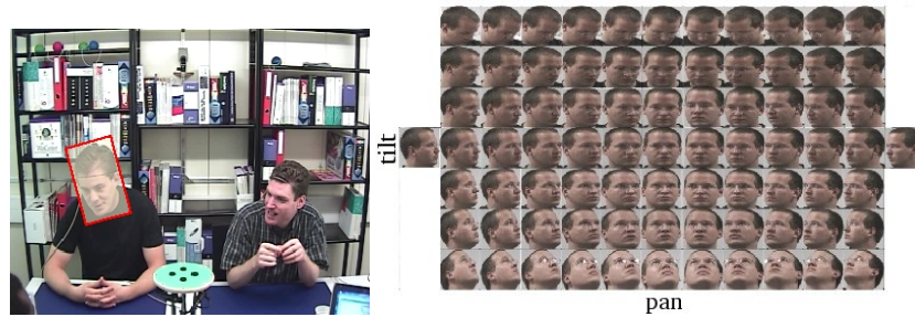
Fig. 6 Head pose extraction. The head localization (position, scale, in-plane rotation, cf left image) and head pose (discrete index indentifying a specific out-of-plane rotation, cf right image) are jointly tracked (taken from (Ba and Odohez, 2008b)).
