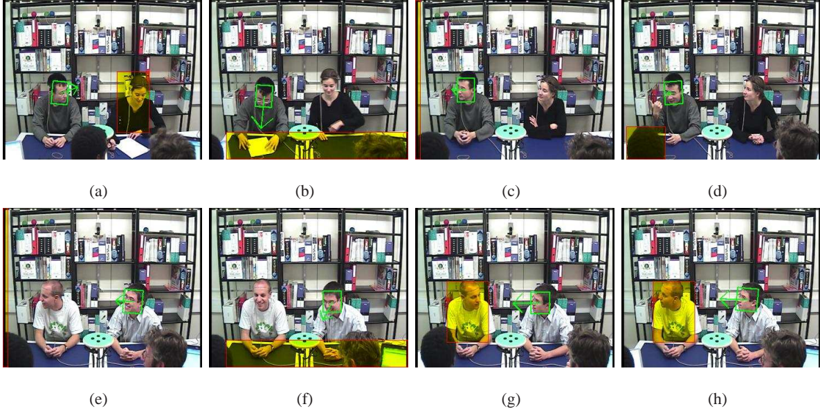
Fig. 9. Example of results and focus ambiguity. In green, tracking result and head pointing direction. In yellow, recognized focus (hmm-ad condition). Images (g) and (h): despite the high visual similarity of the head pose, the true focus differ (in (g): PL; in h: SS). Resolving such cases can only be done by using context (speaking status, other’s people gaze, slide activity etc).
