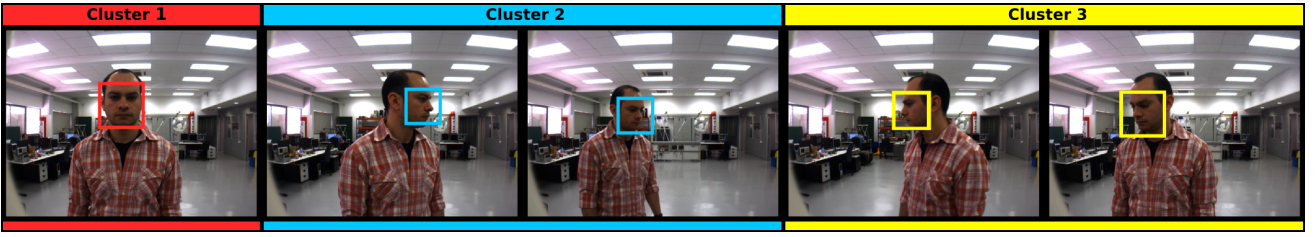
Fig. 1 Example images showing face detection and pose estimation using Random Clustering Ferns (RCFs). The output of RCFs are shown by squared boxes (face detections), whereas the color of each box indicates the face pose. The proposed method is able to simultaneously detect faces and distinguish three different intra-class appearances (face views).
