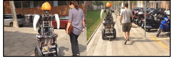
Figure 13: Online learning and detection of objects while the robot navigates in urban areas.
