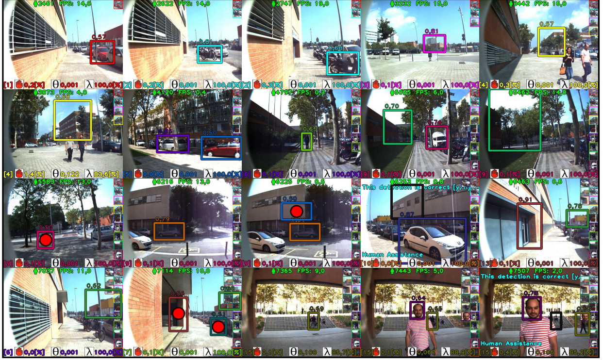
Figure 14: Learning and detection results of the proposed method in urban scenarios. The method is able to compute efficiently multiple classifiers, each one specialized in an object (colored boxes). Black boxes are detection hypotheses assigned to the background class by the human user, while red circles denote false positive detections committed by the classifiers.
