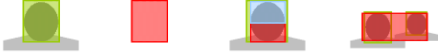
False negative ( FN ) False positive ( FP ) Multiple trackers ( MT ) Multiple objects ( MO )
