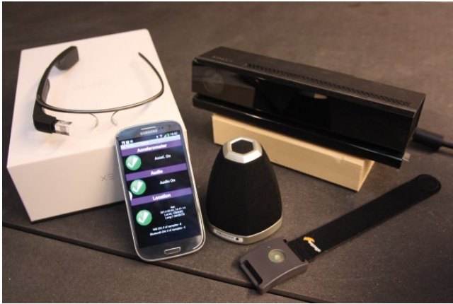
Fig. 2. Devices often used for social sensing (from left to right): Google Glass, Samsung Galaxy SIII smartphone, Dev-Audio Microcone, Microsoft Kinect, and Affectiva Q-Sensor (for physiological data).
