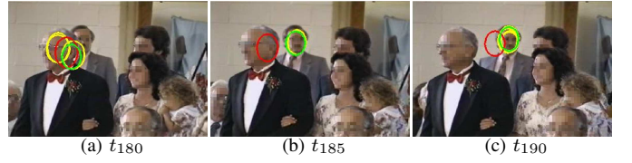
Fig. 12. Head tracking sequence 2 ( N_s=500 ): failure case with the color-based tracker M1.
