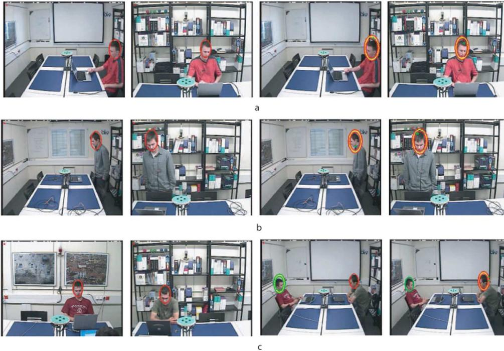
Fig. 7. (a) Tracking a single speaker in the stationary case, and (b) the moving case. (c) Tracking two speakers in the overlapping speech case. The speakers are tracked in each view and displayed with an ellipse. A “+” symbol indicates audio location estimate. A contrasting tone ellipse indicates when the speaker is active.
