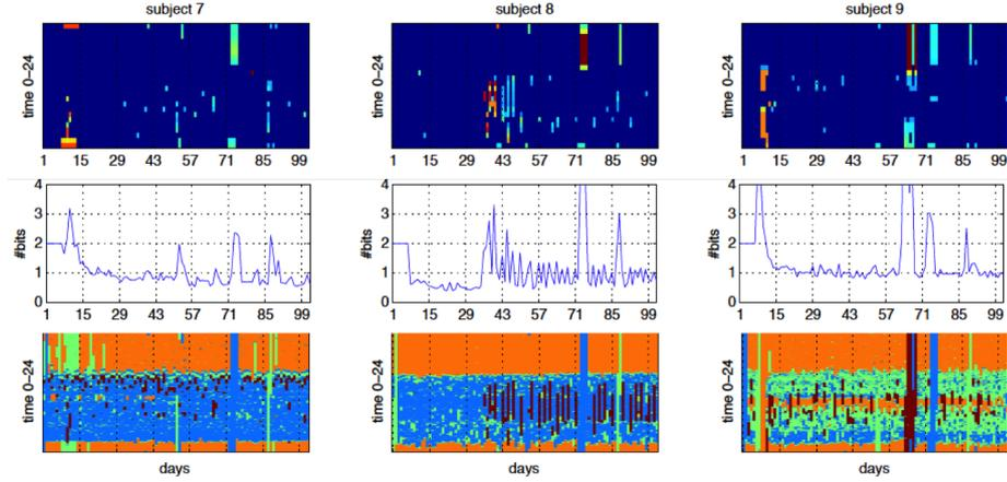
**Fig. 4.** Anomaly scores on three sample subjects. The figures in the first, second and third rows correspond to scores per hour of the day, scores per day, and the mobility pattern, respectively. For the per hour of the day results in the first row, the anomaly score increases from dark blue to dark red. For the mobility pattern, blue corresponds to living room, green corresponds to bathroom, orange corresponds to bedroom, and red corresponds to outings.
