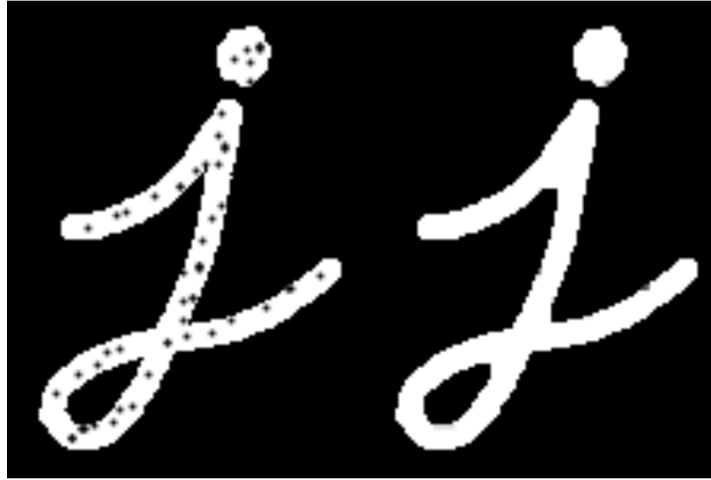
Figure 2.3: opening: erosion followed by dilation ( OpenCV documentation)
