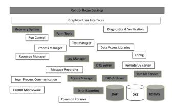
Figure 1: Main components of the controls and configuration software. The figure also indicates dependencies: low level libraries at the bottom and are used by the higher software layers. The elements depicted in grey are components which did not exist or had not been implemented in the original design.
