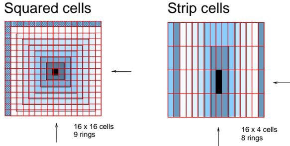
Figure 1: This figure exemplifies ring construction for two type of layers from the calorimeter. The energy peak is marked in black and indicated by arrows.
