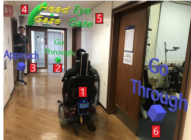
Figure 1: Virtual Reality User Interface . Composite image of the visualizations rendered on the user’s view through the AR headset (1). The affordance Go Through associated with a door was selected by the user and is shown in green (2). The affordance approach associated with a person was not selected and therefore is shown in purple (3). The cursor and timing bar (4) give feedback to the user during the aiming and selection stages respectively. Two different aiming methods can be selected by the user using an on-board menu (5). Some affordances are saved for future usage (6).
