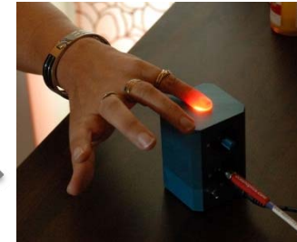
Skin Spectroscopy sensor designed at the University of Vaasa, Finland
