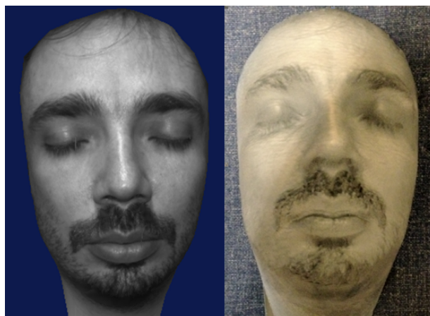
Figure 3: Left: a 3D model generated from point cloud, Right: its corresponding back&white mask made by a 3D printer.
