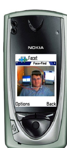
Figure 3. Viola-Jones face detection running on a Mobile Phone. The table on the right shows the processing time (including capture, face finding and display) on several architectures.
