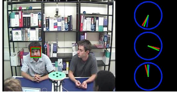
Figure 5: Snapshot of the output of the current head pose tracking system. The three clocks indicates the angle of out-plane (pan and tilt) and in-plane (roll) rotations.
