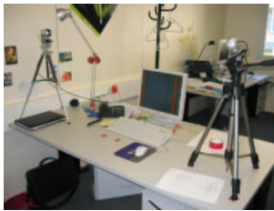
Figure 2: The setup: two synchronized USB webcams.
