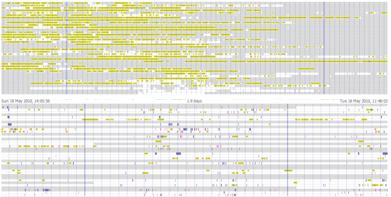
Figure 4: Top: Timeline showing user participation (white) and GPS points (yellow). Bottom: Zooming-in (thin vertical lines represent hours) and superimposing calls/texts shows gaps in the GPS record and the associated difficulty in georeferencing calls.
