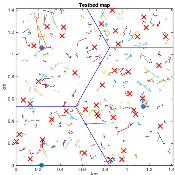
Fig. 2. BS positions in a 2 km<sup>2</sup> map. 3G and 4G are co-located in the centre of each cell, while WiFi APs are placed uniformly (x). The mobility trajectories of the clients are also shown.
