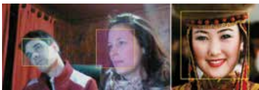
Figure 10: Our real time face detector detects multi-pose faces and labels gender (pink for female, bluish for male) in adverse conditions (left). It also outputs 22 precise facial features, in multi-pose conditions (right).
