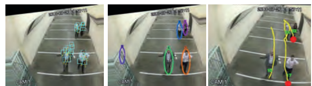
Figure 13: Illustration of the bobbing. During motion, people shoulder move up and down (as well as left and right) according to the gait pattern. Analysis of their visual motion (extracted from their body parts) provides information about the gait frequency as well as when the heel strikes the floor (red dots on the right image).
