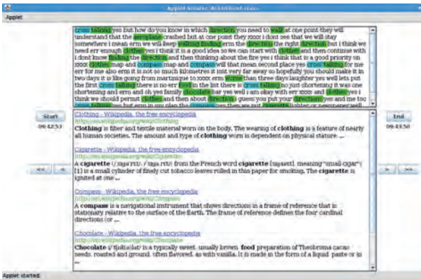
Figure 23: Keyword extraction from a conversation transcript (real-time ASR fragment, top frame) and Wikipedia pages retrieved based on these keywords (bottom frame). When hovering over one result, the corresponding keywords change from green to blue.
