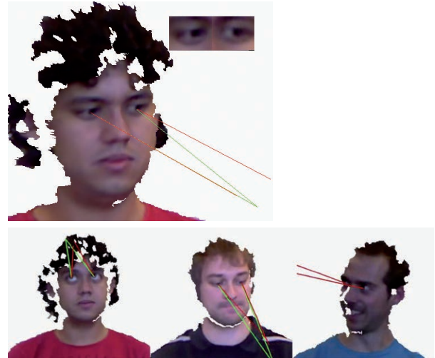
Figure N°6 : Top: 3D rendered mesh from depth and RGB image. Left top: using the 3D tracker output, eye regions from the RGB image can be cropped and rendered as if the head pose was frontal. Bottom: sample of recognized gaze under free head movements. Green lines materialize the ground-truth gaze directions, while the red ones represent estimated gaze.
