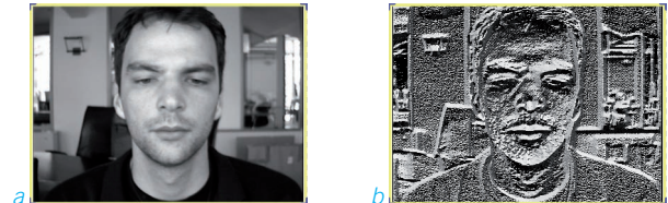
Figure 9: Illustration of the LBP feature map (b) for the original image (a).
