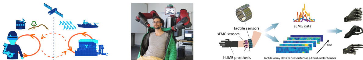
Figure 17: Human-centric robotic applications. Left: Teleoperation assistance for the control of a bimanual robot (DexROV project), where the robot assists the teleoperator when repetitive or structured tasks are detected, as a form of human-robot collaboration. For example, if the robot observes that the task of drilling requires the drill to be perpendicular when it approaches a surface, the robot will then automatically orient the drill when it approaches another surface, letting the teleoperator concentrate on the position to drill while letting the robot maintain the correct orientation. Center: Personalized assistance in dressing (I-DRESS project), where the robot learns by demonstration the preferences and type of assistance required by each user. This is achieved by extending the movement primitives frequently employed in robotics to a wider repertoire of skills composed of reactive behaviors based on force, impedance, position and orientation. Right: Online learning and adaptive control of a prosthetic hand (TACT-HAND project), where electromyography and tactile sensing data are combined to control a prosthetic hand.
