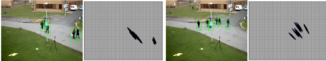
Figure 7: Person detection obtained with a deep neural network, and the corresponding occupancy map estimates.
