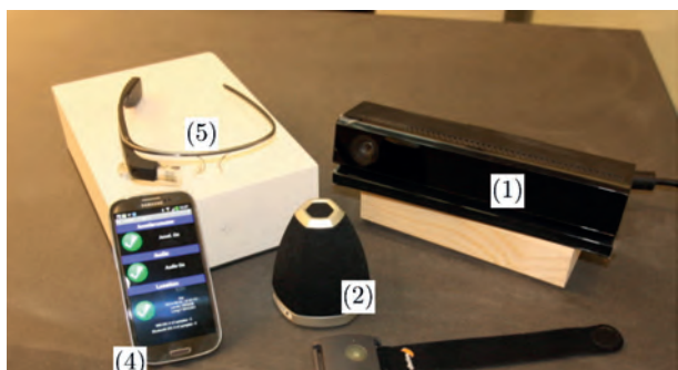
Figure 8: Sensors available in the social sensing lab. (1) Kinect V2, (2) Microcone, (3) Q-Sensor, (4) Android smartphone, (5) Google Glass.
