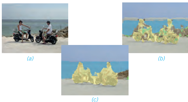
Figure 16: Our recurrent scene parser over original image (a) segments the image as shown in (b). Due to its recurrent nature, it can be fed again with its own prediction (b) and the original image (a), which leads to (c): most mistakes are corrected.
