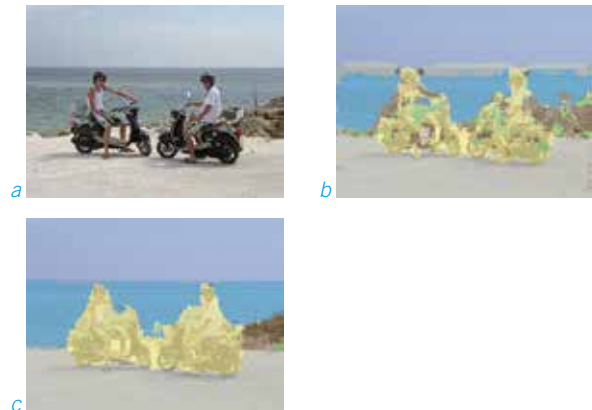
Figure 9: Our recurrent scene parser over original image (a) segments the image as shown in (b). Due to its recurrent nature, it can be fed again with its own prediction (b) and the original image (a), which leads to (c): most mistakes are corrected.
