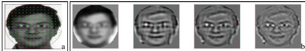
Figure 8: (a) Grid for feature computation. (b) Left-to-right: filtered images by a Gaussian and three Gabor wavelets.
