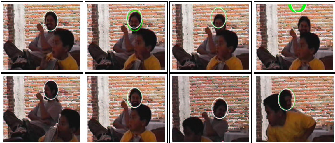
Figure 4: Head tracking 1. Top row: shape tracker, frames 9, 11, 13, and 15. Bottom row: shape+correlation tracker, frames 1, 15, 39, and 63.
