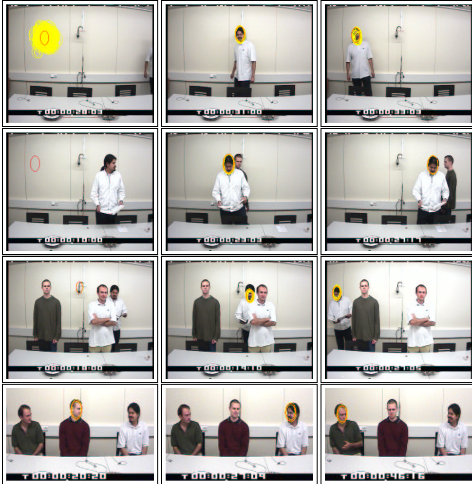
Figure 6: AV tracking. Mean in red, standard deviation from the mean in yellow. First row: Walk . Second row: Visual Clutter . Third row: AV occlusion . Fourth row: Chat .
