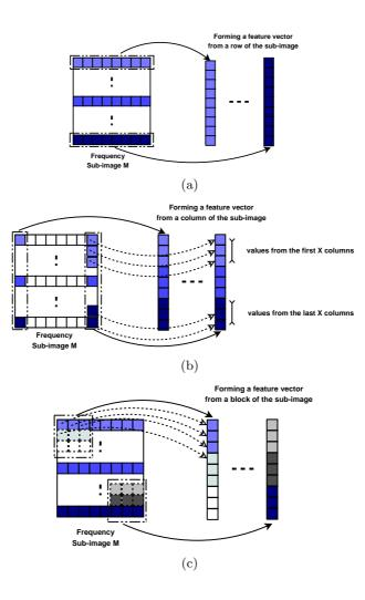
Fig. 3. Forming the feature vectors (a) along the row of the frequency sub-image, (b) along the columns of the frequency sub-image and (c) using blocks of the frequency sub-image.
