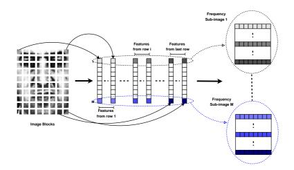
Fig. 2. The figure above describes how the face can be decomposed into separate frequency sub-bands (sub-images).
