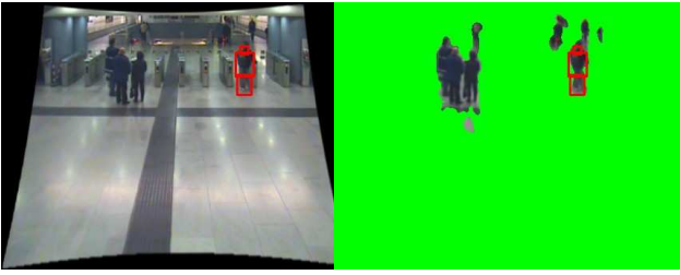
Figure 2: The 3 bounding boxes associated with a projection of a body model. Left: displayed on the original image (after distortion removal). Right: displayed on the foreground image. To build the color histogram observations, only the visible foreground pixels are taken into account.
