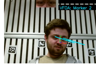
Figure 4: Gaze estimation example showing: head pose (red-green-blue coordinate system on the nose); gaze (cyan rays); extracted and exploited eye images after frontalization (top, together with the VFOA estimate).
