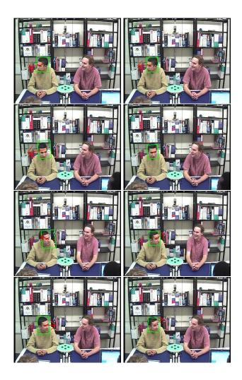
Figure 5: Sample of tracking failure for MSPF due low number of samples. First column: MSPF; Second column: RBPF.
