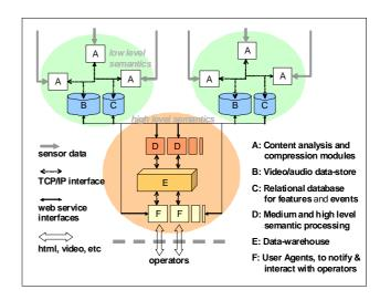
Figure 2: Diagram to illustrate the likely design configuration for the real-time subsystem.
