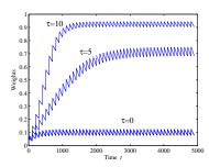
Figure 1. Evolution of a mode weight for a quasi-periodic pixel x, where the data repeatedly match the mode for 10 frames, and don't match the mode for the subsequent 90 frames ( $\alpha_w =$ 0.005,  $w_{init} = 0.01$ ), with different constants  $\tau$ .
