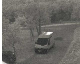
*Scene measured in the 1.4–1.8  $\mu\text{m}$  spectral band on a moonless night (© Onera 2010)*
