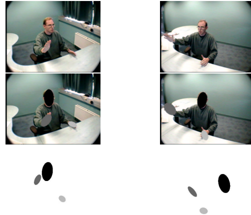
Fig. 1. Top: left and right captured images. Middle: left and right images with projected ellipsoids. Down left: ellipsoids projection on the frontal plane. Down right: ellipsoids projection on the side plane (the cameras are on the left side).
