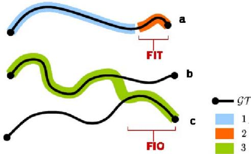
Figure 10: Types of identification errors. Three objects are tracked by three estimates. A falsely identified tracker error (**FIT**) occurs when object  $a$  is tracked by a second estimate,  $\mathcal{E}_2$ . A falsely identified object error (**FIO**) occurs when an estimate swaps ground truths ( $\mathcal{E}_3$  swaps from  $\mathcal{GT}_b$  to  $\mathcal{GT}_c$ ).
