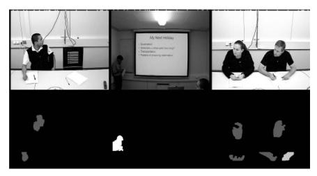
Fig. 3. Blob extraction in the multicamera meeting room. The top row of images shows a frame from each of the three cameras, and the bottom row shows the detected skin blobs (left and right) and moving blobs (center).
