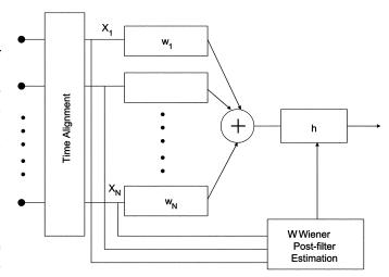
Fig. 3. Speech enhancement module with filter-sum beamformer followed by a postfilter.
