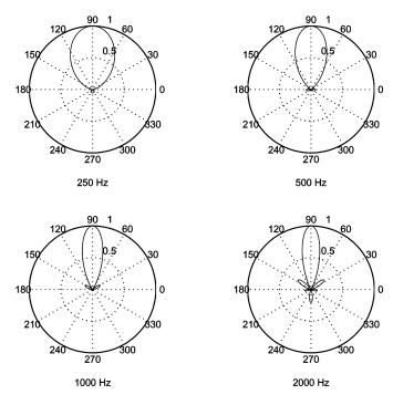
Fig. 4. Horizontal polar plot of the near-field directivity pattern  $(r=1\ \mathrm{m})$  of the superdirective beamformer for an eight-element circular array of radius 10 cm.
