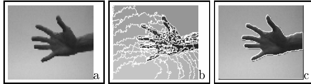
Fig. 1. SVO extraction operator. Hand sequence. (a) Original image \mathbf{I}^1 . (b) Partition P^1 (segmentation model superimposed); (c) SVO partition P_{SVO}^1 = \psi(P^1) (original image superimposed).
