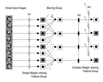
Figure 2. Inherent Rotation invariance is gained by deploying weight-kernel sharing feature groups (both simple and complex) as well as orientation blurring layers.
