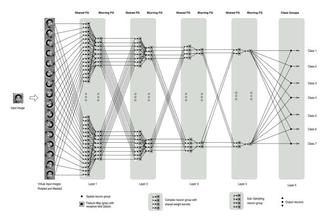
Figure 1. Extended Neoperceptron Architecture: The network consists of two stages: virtual input image generator followed by a convolutional neural network with shared feature groups (Shared FG) and blurring feature group (Blurring FG) layers.
